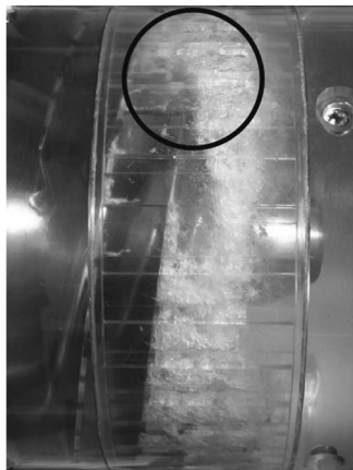
Fig. 12 Tip cavitation in the inducer in the case with JG2(40,20) for \phi=0.078 and \sigma=0.050
