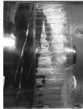
Fig. 18 Tip cavitation in the inducer in the case with JG3(40,10) for \phi=0.078 and \sigma=0.050
